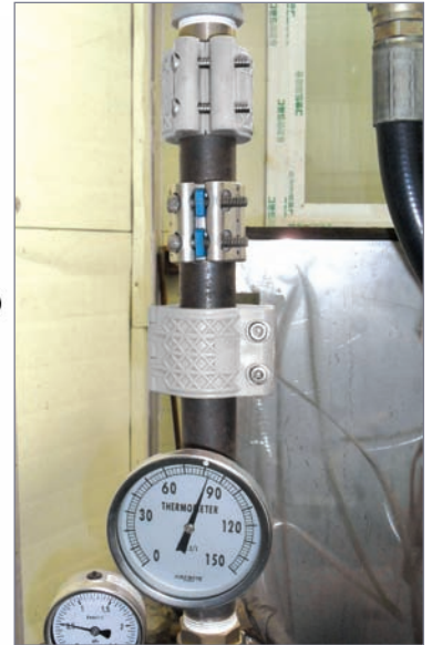
80°C × 30min. × 20kg/cm 2 High-temperature circulation test
