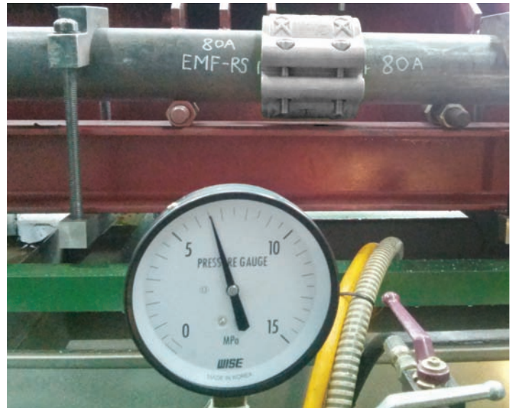
80A 6.5Mpa (65kg/cm 2 ) Pressure Test
