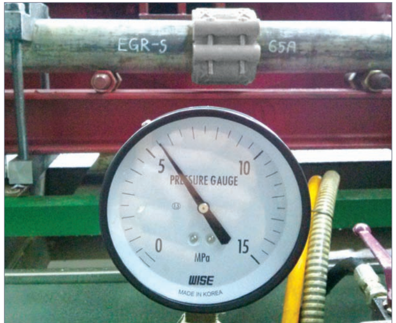
65A 5.5Mpa (55kgf/cm 2 ) Pressure Test
