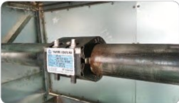
▲ The product just before the fire test, after being installed in a furnace
