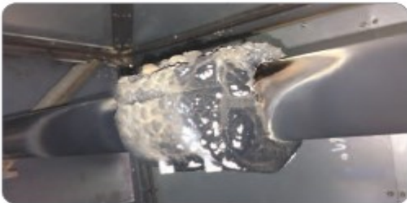
▲ The product after completion of the test with normal pressure being maintained at over 800°C
