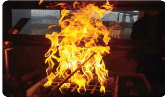
Test Details : A fire resistance test was conducted for 30 minutes at 800°C. (Pressure of 18kgf/cm 2 maintained) Test Regulations : ISO 19921, ISO 19922
