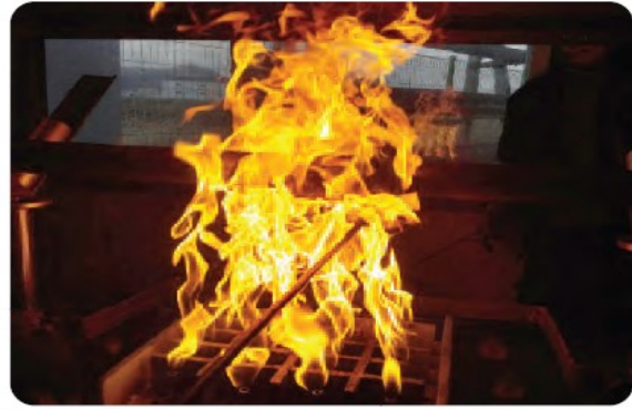
Test Details : A fire resistance test was conducted for 30 minutes at 800°C. (Pressure of 18kgf/cm 2 maintained) Test Regulations : ISO 19921, ISO 19922
