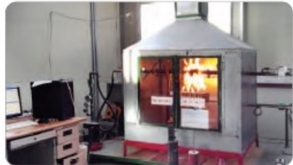
▲ The product during the fire test according to ISO 19922 regulation
