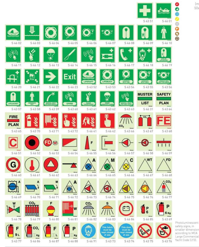
Photoluminescent safety signs, in smaller dimension, according to MCA
